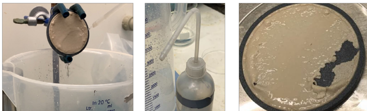
Figure 3 Method for removing external filter cake from formate fluids.
